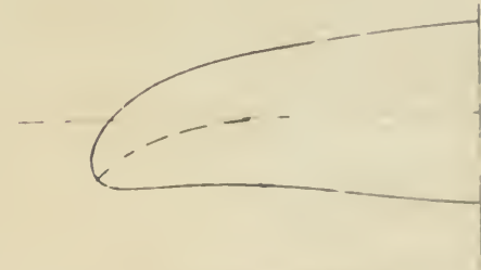
LEADING EDGE NO. 7 ORIGINAL CONTOUR MODIFIED APP. TO 420-- SERIES AIRFOIL REF. DWG. W.T. 179-196 7 OF 7
